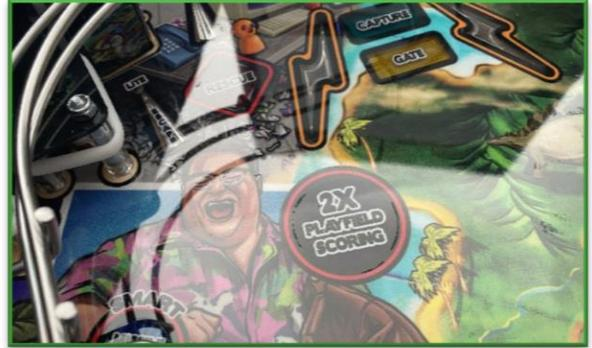
On new pinball machine the clear coat can evaporate which results in these "wet spots". You can easily get rid of them.
